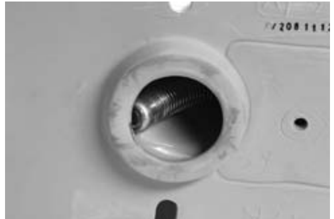
Figure 20 – Camera Head Blocked in Turn
