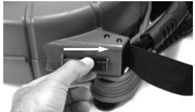
Figure 4 – Unlatching the microDrain Reel Case
