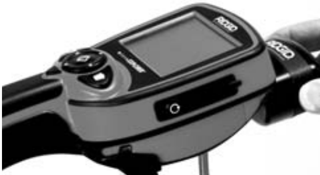
Figure 10 – Connecting the microEXPLORER Camera Monitor
