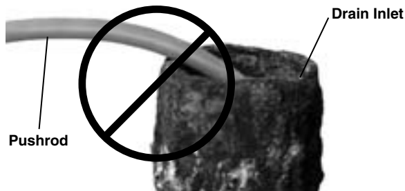
Figure 18 – Avoid Pulling At Sharp Angles
